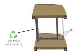
**E:** Using a #2 Philips screwdriver, remove the end frame and seat extension from the seat frames. On double or triple seat configurations you will need to do the same with the center arms. Place the seat frame and seat extension to one side.
